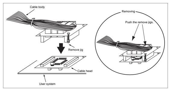
Figure 4 Fastening Cable Body
